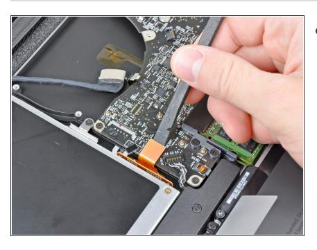
Use the flat end of a spudger to pry the optical drive connector up and out of its socket on the logic board.
