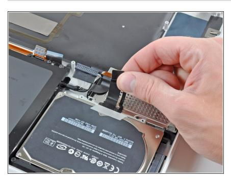
Peel the hard drive and battery indicator cables off the adhesive securing them to the express card cage.
