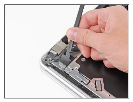
Use the flat end of a spudger to peel the thin plastic cover off the top and sides of the Bluetooth board housing.
