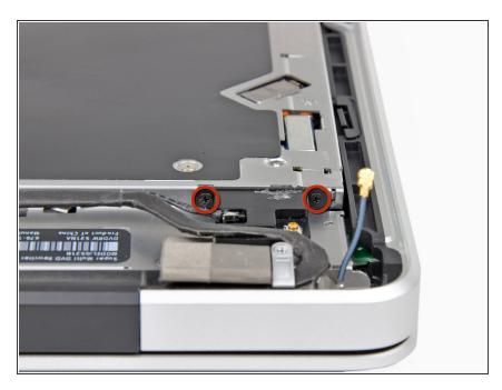
Remove the two 2.2 mm Phillips screws securing the Bluetooth housing to the side of the optical drive.
