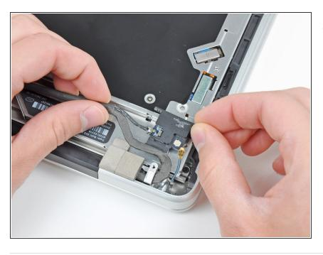
De-route the camera cable from its slot in the Bluetooth housing and remove the Bluetooth board from the upper case.
