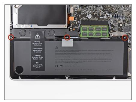
Remove the three 6.5 mm Tri-point screws securing the battery to the upper case.
