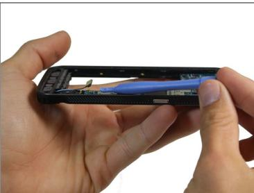
• Use your finger or a plastic opening tool to disconnect the 3 button ribbon cable from the motherboard.
