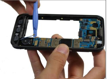
• Use a plastic opening tool to disconnect the the blue wire shown in the picture.
