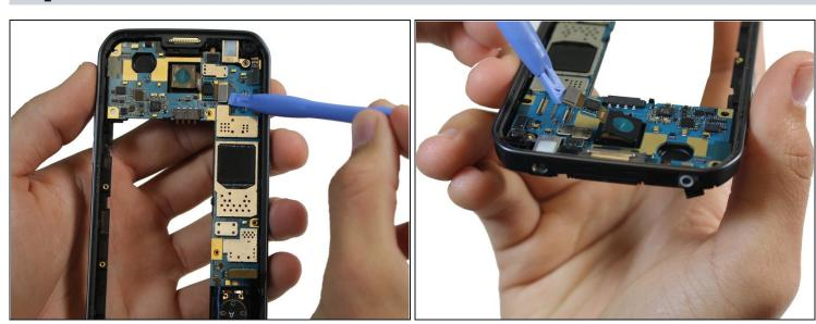
• Use your finger or a plastic opening tool to disconnect the rear-facing camera from the motherboard.
