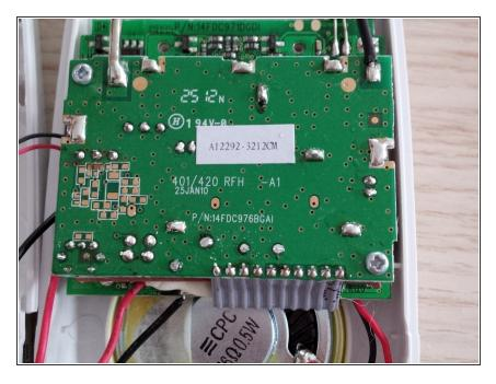
remove the 2 PCB's by removing the screws shown in the picture.
