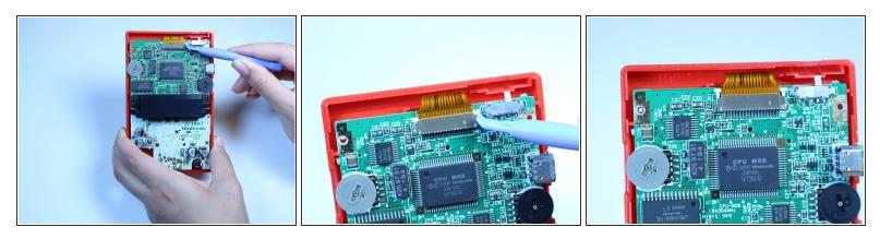
• Use a plastic opening tool to dislodge and remove the clip securing the ribbon cable.
