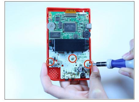
Use a Phillips #1 screwdriver and turn counterclockwise to remove the three screws on the motherboard.
