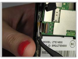
• Use the tweezers to remove the four ribbon wires on the sides of the device.
