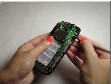
Gently pry the mid frame away from the rest of the phone to expose the motherboard.
