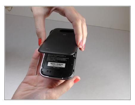
Remove the back cover of the phone to expose the phone's midframe.
