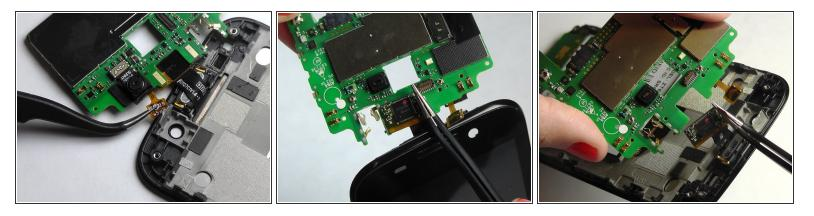
Remove the connector to free the motherboard from the screen.
