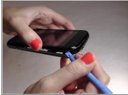
Wedge the flat end of the spudger between the mid frame and the digitizer.
