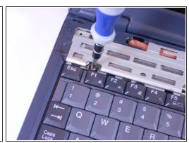
• Using an Phillips screwdriver, unscrew and remove two screws labeled B2.6.
