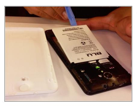
Remove battery with plastic opening tool.
