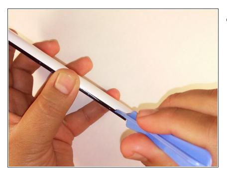
Remove the back cover on the phone with the plastic opening tool.
