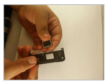
Remove the speaker from the backing of the speaker holder.
