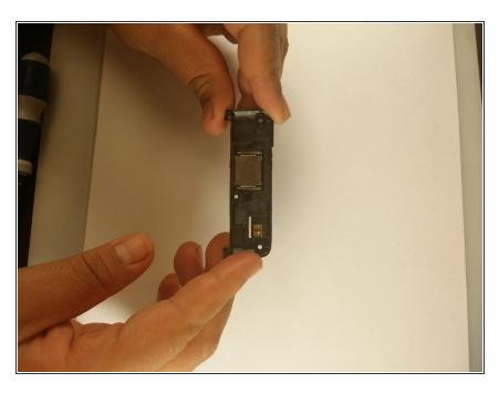
After removing screws gently pull off the speaker from the back of the phone.
