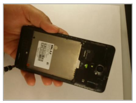
On the bottom part of the back of the phone with a Phillips screwdriver #00 tool remove the 6 screws that hold the speaker in place.
