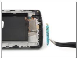
Use a pair of tweezers to carefully pry up and remove the daughterboard at the bottom end of the screen assembly.
