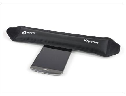
Apply a heated iOpener to the top end of the screen to loosen the adhesive underneath.
