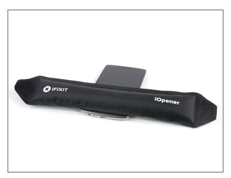
Apply a heated iOpener to the bottom end of the screen to loosen the adhesive underneath.
