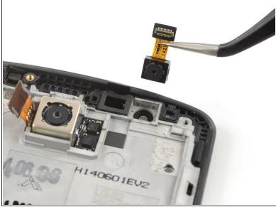
Use a pair of tweezers to remove the front camera.
