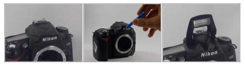
• Use a plastic opening tool to lift up the flash.
