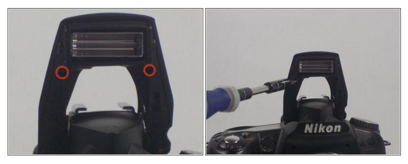
• Using a PH00 screwdriver, remove the two 5.3 mm Phillips screws from the flash casing.
