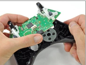
• Lifting from the headphone jack and power plug, remove the logic board from the front case.
