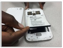
Remove the back cover by lifting at the notch towards the bottom of the phone. Use your fingernail to pry up.
