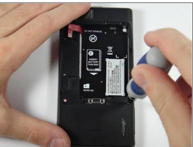
Remove the circled screws using a T-5 torques. These screws will be 4.3 millimeters in length.
