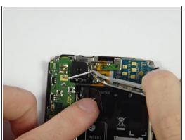
Using tweezers, remove the white wire at the top of the phone near the camera.
