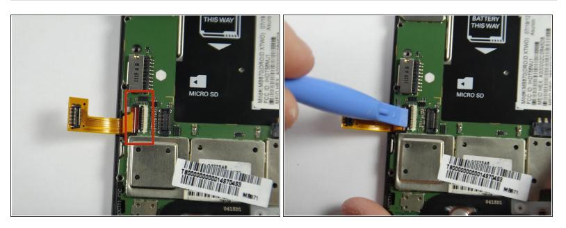
Using a pry tool, lift the jawbone connector.
