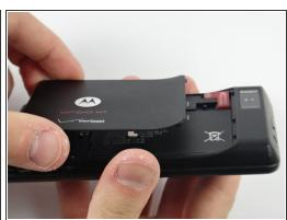
Slide the plastic case off of the back of the phone, exposing the battery.
