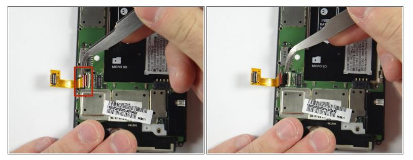
Using tweezers, carefully disconnect the cable connector by pulling the cable out.
