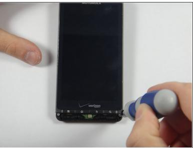
Remove the circled screws using a T-5 torques.. These screws should be 5.8 millimeters in length.
