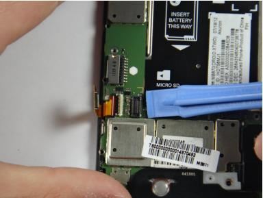
Using the plastic opening tool, lift up to remove the connector.
