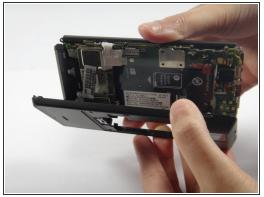
Using a plastic opening tool, snap open the phone. It should separate into a front piece with the hardware and a plastic backing.
