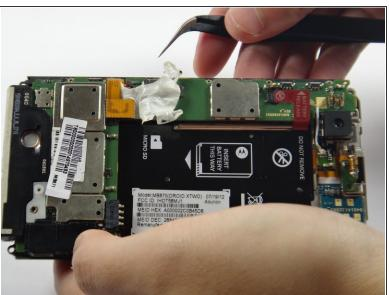
Using tweezers, removed the white electrical tape on the motherboard.
