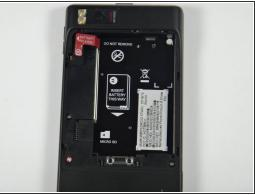
Pull up on the red battery release tab and pull the battery out of the phone.
