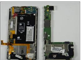
Using a spudger, remove the camera. Lift up the motherboard and slide the spudger under the camera.
