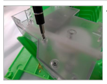
Remove five screws (1.5 cm in length) using a Phillips #00
