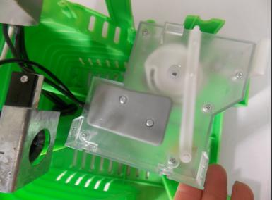
There are four screws (circled in red) that need to be removed with a Phillips #00 Precision screwdriver.
