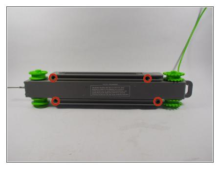
• Remove the four exterior screws
