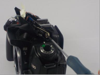
Using a PH00 screwdriver, loosen the 3.3 mm Phillips screw from the spring.
