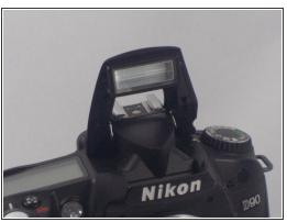
Use a plastic opening tool to lift up the flash.
