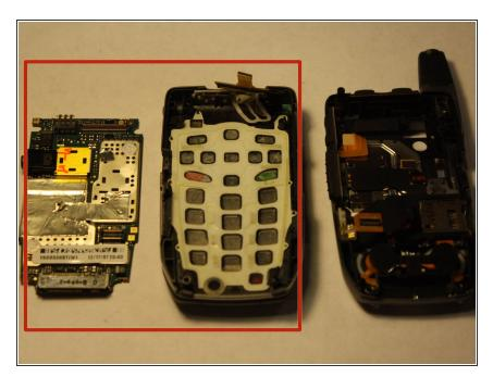
Insert new logic board and reattach top right cable.
