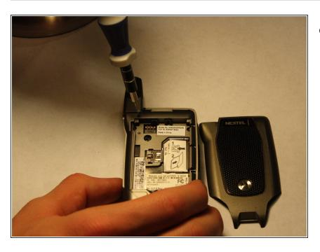
Snap the front and back of the phone back together and reinsert screws 1 through 4.
