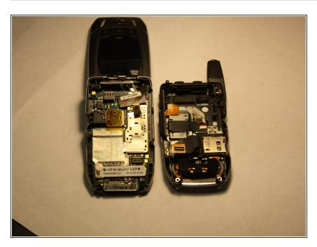
Once all four screws are removed, you should be able to take off the back half of the phone.
