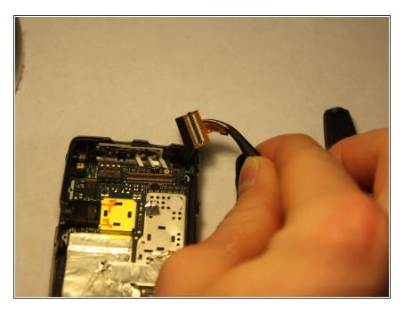
Remove the connection at the top right of the circuit board.
