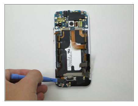
Use the narrow plastic tool to pry up the black foam covered rectangular connector.
