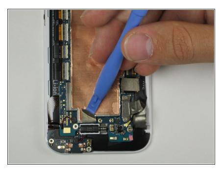
Starting from the copper plate, peel up all three woven, silver colored tapes using the spudger or narrow pry tool.
