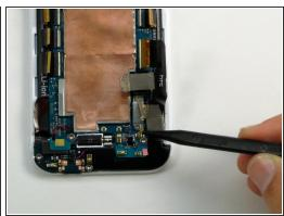
Use the pointed end of the spudger to pop off the four antenna connectors. Three are located on the top left corner of the motherboard and one on the bottom right.
