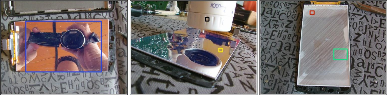
**i** I used a hair dryer with cold air to help to separate the layers.
