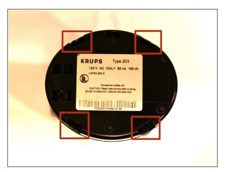
In each of the four rectangular slots on the bottom of the device, there is an E-shaped clip.
