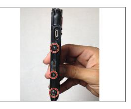
• Remove the eight 2.5mm Phillips #00 screws in the holes of the casing.
