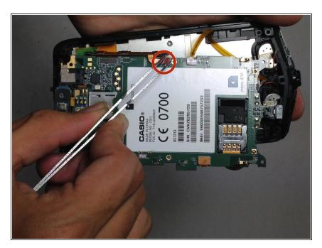
Following step 6, remove the adapter connecting the volume buttons to the motherboard.
