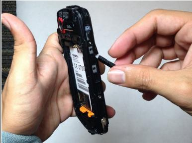
Following step 4 in the prerequisite guide, remove the volume pads located on the side of the phone with a gentle pull.
