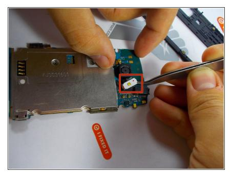
• The white rectangle with the yellow square is the flash. Gently lift up and disconnect flash module. Take your new flash and aligning the connection point to the connection hole, push it down firmly until it is snug in place. Follow the steps backwards to put phone back together.
