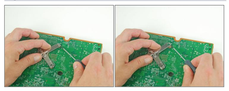
(i) Rotate the logic board 180 degrees counter-clockwise.
