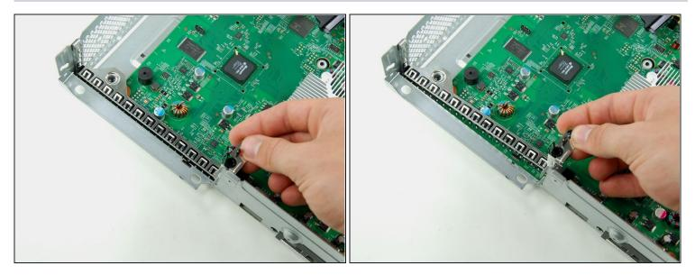
• Lift the optical drive retaining bracket off the logic board.
