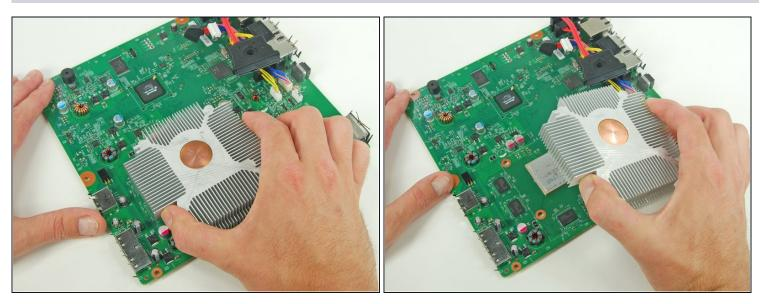
i Using one hand to hold the heat sink in place, carefully turn the logic board over.
