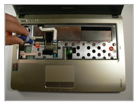
Unscrew the two M2X3 screws that were under the keyboard.
