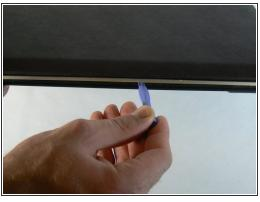
Use the blue plastic opening tool to pry the silver plastic keyboard surround out from the black plastic bottom. You will need to do this around the entire perimeter of the laptop and will hear a pop every time one of the retention clips is unlatched.
