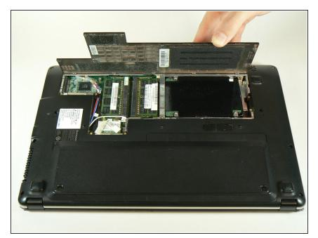
Lift the back panel from the side closest to the battery and remove the panel.
