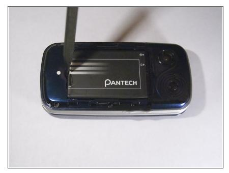
Carefully lift the battery up from where the spudger is pointed.
