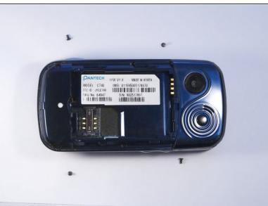
Use a PH000 screwdriver to remove the four 2 mm screws from each corner of the device.
