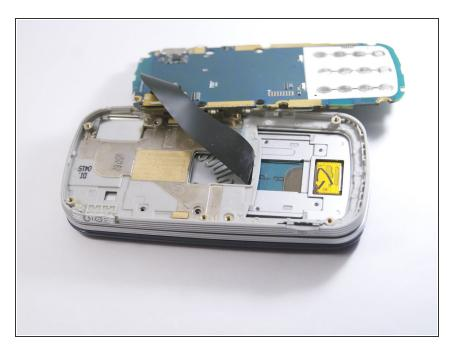
Carefully lift up the motherboard to expose the volume button.
