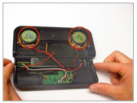
Locate the two individual speakers on either side of the front cover.
