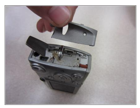
Remove the right side cover from the camera casing.
