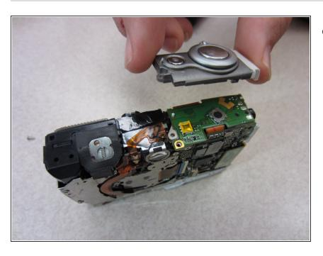
Gently remove the shutter button unit from the rest of the camera.
