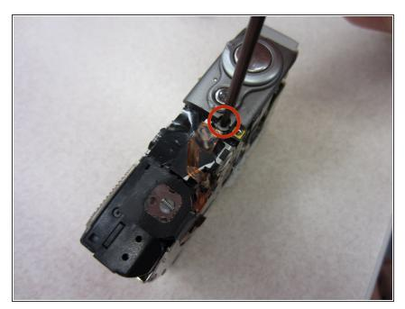
Unscrew one .235 inch long Phillips screw using a #00 Phillips screwdriver from the top of the camera.
