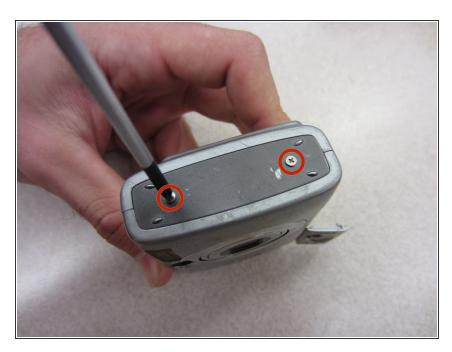
Remove two .085 inch Phillips screws from the left side of the camera using a #00 Philips screwdriver.
