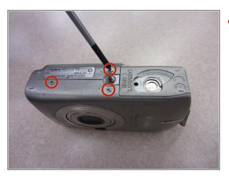
Remove three .15 inch Phillips screws from the bottom of the camera using a #00 Phillips screwdriver.
