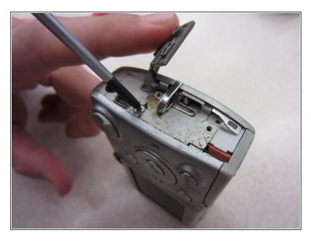
Remove a .07 inch Phillips screw using a #00 Phillips screwdriver.
