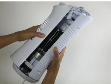
Pull the front and back parts of the case away from each other until the back is free from the front.
