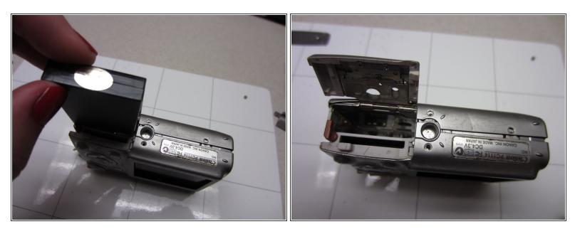
Slide the battery out of the battery compartment.
