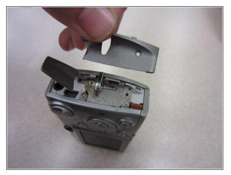
• Remove the right side cover from the camera casing.
