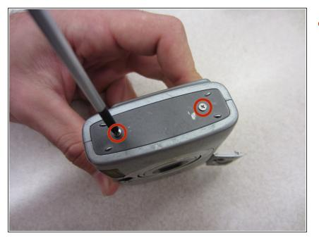
Remove two .085 inch Phillips screws from the left side of the camera using a #00 Philips screwdriver.
