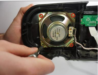
Use a 14cm Phillips #1 screwdriver to remove the four respective screws attaching the left and right speakers to the front panel.
