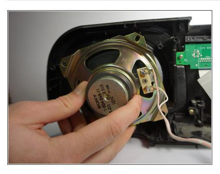
Remove the speakers from the front panel.
