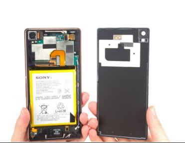
Slide the guitar pick to cut the sticker and remove back cover.
