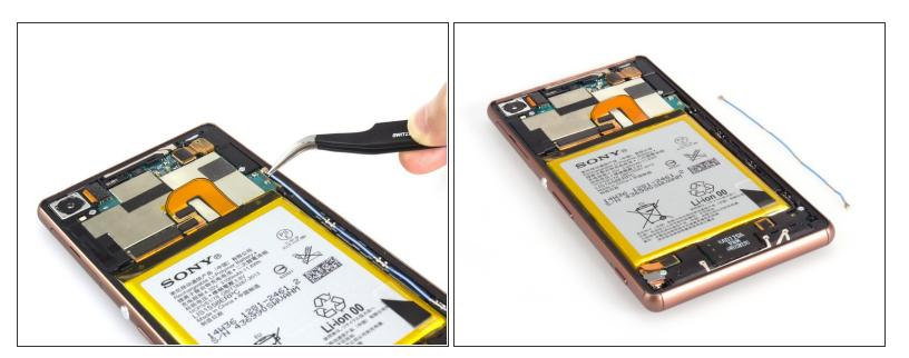
Remove the signal flex finally. But it's hold tightly, please handle it carefully.
