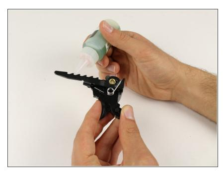
Place two to three drops of oil on the ridged area of the firing mechanism.
