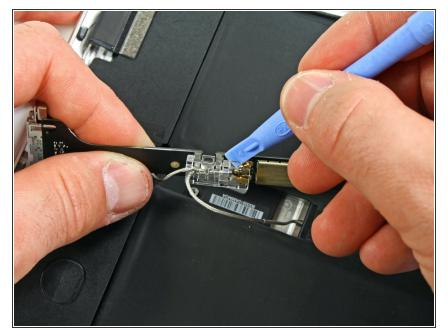
Using an iPod opening tool, carefully remove the plastic cover shielding the WiFi/Bluetooth board and dock connector cable.
