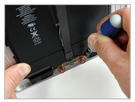
Remove the two 2.84 mm T5 Torx screws securing the dock connector cable to the rear case.
