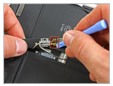
Carefully pry the Wi-Fi and Bluetooth antennas up from their respective sockets on the Wi-Fi/Bluetooth board.
