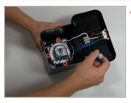
Remove the three 60mm Phillips size 0 screws holding the top cover on.
