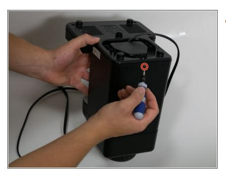
Remove the single black Phillips size 0 10mm length screw on the back of the machine.
