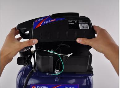
Remove the plastic shroud from the compressor.
