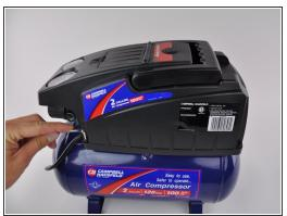
Unscrew the four 1cm long shroud screws using a 6mm Allen Wrench.
