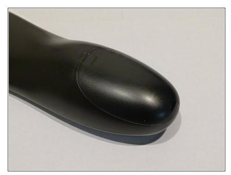
On the back bottom of the controller, a housing holds the batteries that are used to power the controller.
