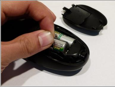
Carefully pull the black tap to remove the batteries from the battery housing. When inserting new batteries, be aware of the correct orientation.
