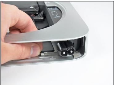
• Pull the silver metal AC-In socket retainer away from the side of the outer case and remove it from the mini.
