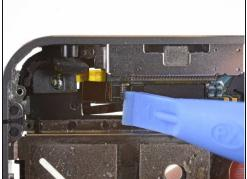
Use the edge of an iPod opening tool or your fingernail to lift the home button ribbon cable retainer.
