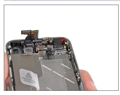
Remove the 1.5 mm Phillips screw securing the front panel near the headphone jack.
