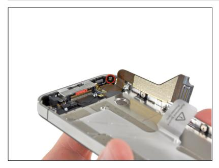
Remove the 1.5 mm Phillips screw near the dock connector ribbon cable.
