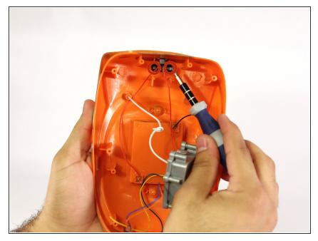
On the top of the inside cover you will see the back side of the on/off switch. Remove the two 7.2 mm Philips #00 head screws holding the switch in place.
