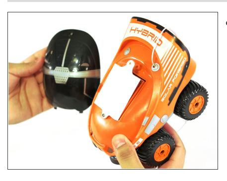
After the screw has been loosened, lift the cover off.
