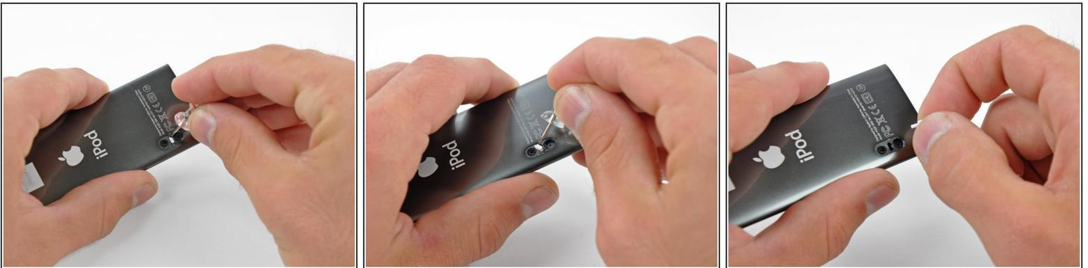
**i** There is a small white retainer between the camera and microphone that keeps the inner components from sliding around.
