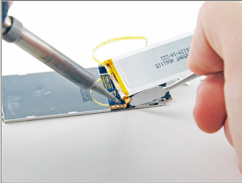
**i** The battery on the Nano is attached via solder pads with small holes that go through the battery ribbon cable and attach to flat pads on the face of the logic board. In this step, you will heat each solder pad individually while using a metal spudger to pry it up from the logic board.
