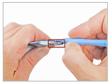
Use an iPod opening tool to pry the hold switch button off of the hold switch plate.
