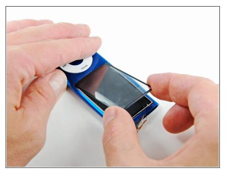
Lifting the glass from the side nearest the top of the iPod, remove the glass panel from the Nano.
