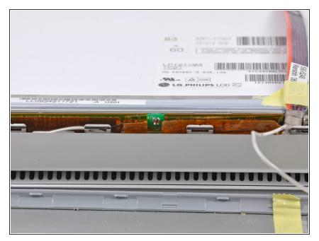
• Remove the Phillips screw securing the inverter board.
