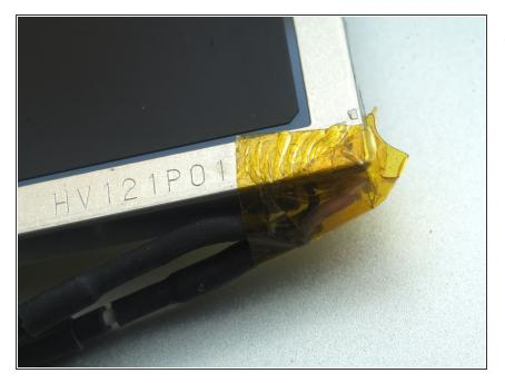
• Apply some electric tape here, to avoid short circuit.
