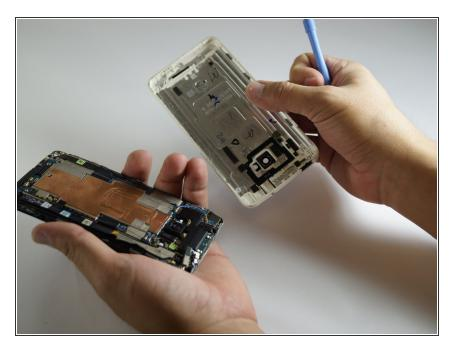
Once the crease has been loosened all around, pry the back panel open and lift until it can be removed.
