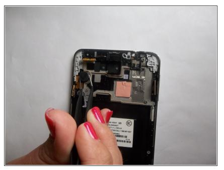
Remove the vibrating motor by pulling up on it carefully with the tweezers.
