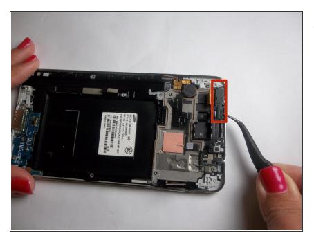
Remove the metal bracket located in the top left hand corner.
