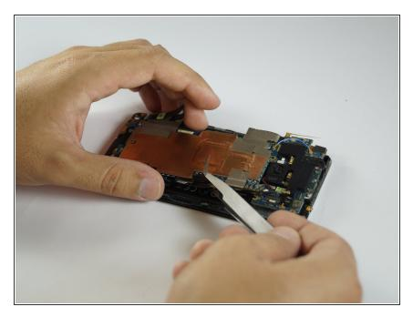
Lift the motherboard completely out of the phone with the tweezers. (may stay attached at the bottom by tape)
