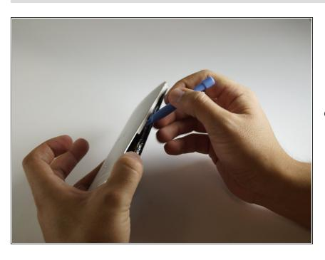
The rear case is held on by glue and eight tabs on the screen bezel. On the volume side there is one above the rocker and three below; on the SIM side all are below the slot. Insert the plastic opening tool between the case edge and the screen bezel, aiming to prise the rear case edge outwards to loosen the glue and free the tabs, one at a time.
