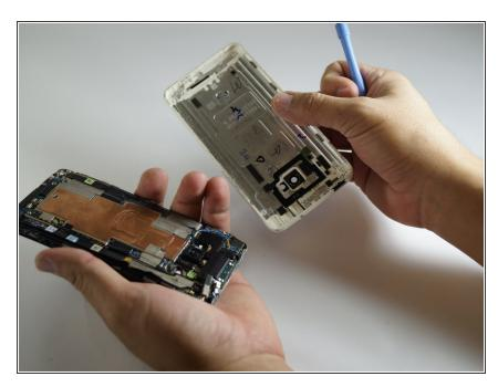
Pry the back open once loose and lift. The back panel will come off with time.
