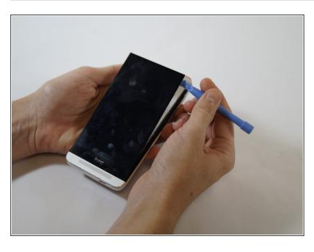
Wedge the plastic opening tool into the crack around the screen on the top, left and right sides.
