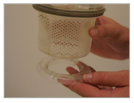
If screen is beyond washing clean or is cracked, connect new screen to cyclone and collar.
