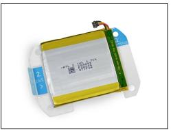
• Grasp the battery with your fingers and pull directly away from motherboard to separate the battery from the display.
