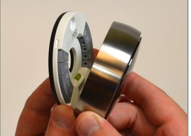
Grasp the display's metal outer ring with your fingers and pull directly away from the wall.
