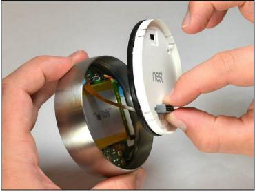
Pinch the gray 20-pin connector with your fingers and pull directly away from the display.
