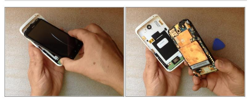
Remove the display assembly from the body of the phone.
